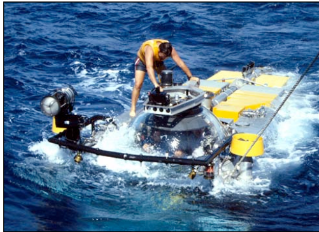
Fig. 5. One of the two Johnson Sea Link submersibles operated by the Harbor Branch Oceanographic Institution. Forward acrylic sphere holds one pilot and principal science observer, aft metal sphere holds a sub crew member and one additional science observer. Maximum diving depth 1,000 m (3,280 ft). Image courtesy of Gregory S. Boland.
